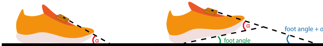
Figure 2. The measured IMU-based foot angle (foot angle + \alpha ) corrected with the mean foot angle ( \alpha ) during the foot flat phase of the first 10 strides, to consider the foot angle during the foot flat phase to be zero degrees.
